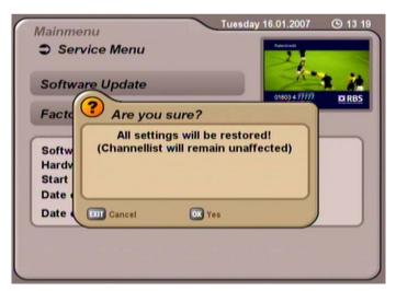
Press the OK button to load the factory default settings. The channels and favourites lists remain unchanged.
